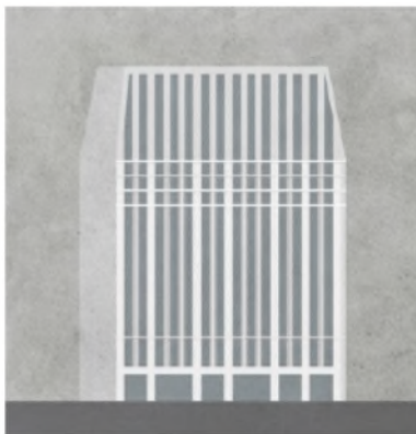
04 Horizontal cornices provide definition to the latticed middle section
